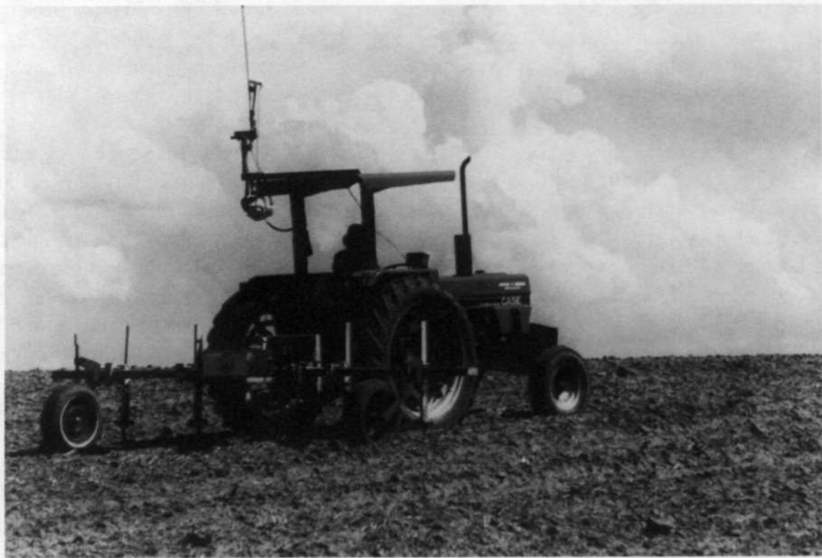
Fig. 1. Photograph of mobile, 'fixed-array' four-electrode system with GPS antenna mounted on the mast.
