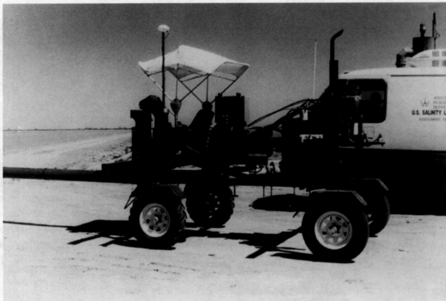
Fig. 5. Photograph of mobile salinity assessment vehicle with combined electromagnetic induction and four-electrode soil conductivity sensing systems.
